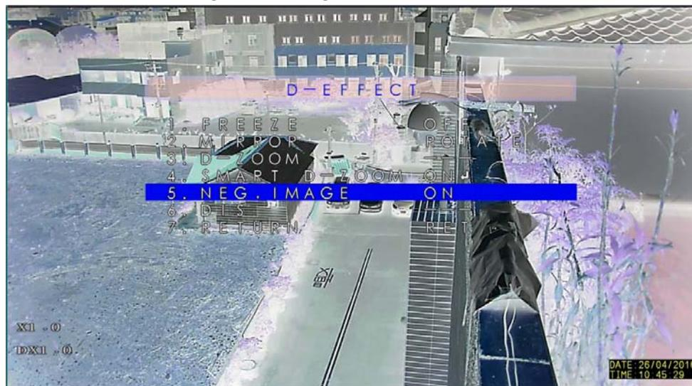
P.S. Negative image is deployed when user do not wish to display the actual color, but actual object shape is required.
