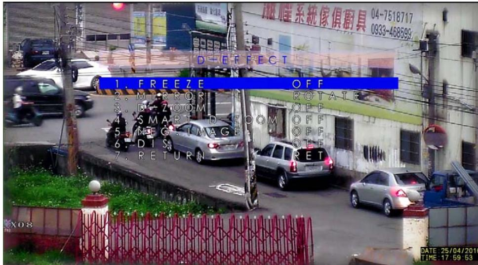
3.6.2.1 FREEZE : Choose ON to freeze on current frame, the camera does not record new frame.
