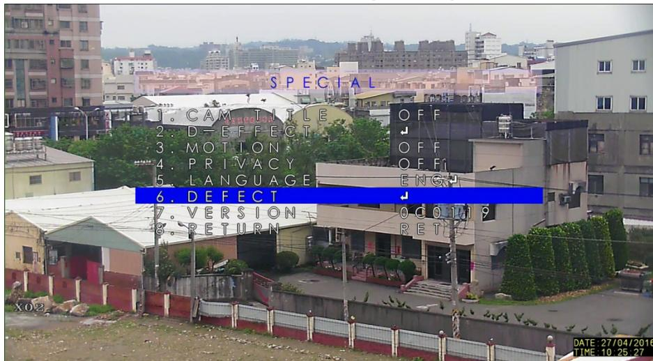
Press ENTER to access defect spot patching settings as below.
